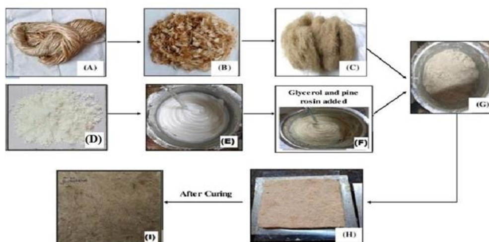
Fig. 1 Fabrication route of biocomposite. (A) Strand of jute fibre, (B) Chopped jute fibre (15 mm), (C) Opened jute fibre, (D) Starch Powder, (E) Preparation of Resin, (F) Resin ready for use, (G) Resin/fibre mixture, (H) Pre-cured biocomposite sheet on mould and (I) Biocomposite after Curing.
