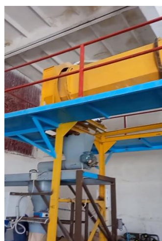
Figure 4. Photos of a manufactured hexagonal mixing drum as part of a pickler of pubescent cotton seeds.
