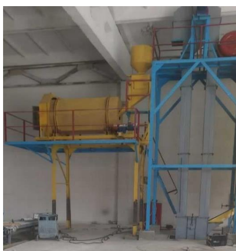
Figure 4. Photos of a manufactured hexagonal mixing drum as part of a pickler of pubescent cotton seeds.
