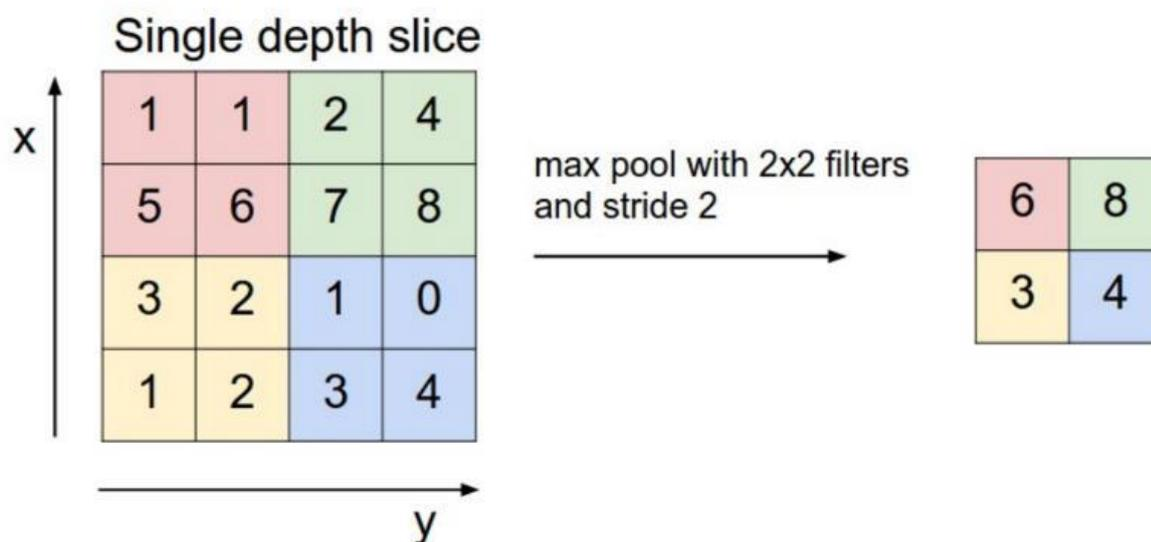
Figure 3: operation of pooling with 2X2 filter
