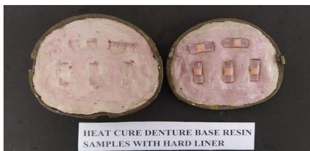
Figure 2 : Heat Cured Denture Base Resin samples relined with Hard liners
