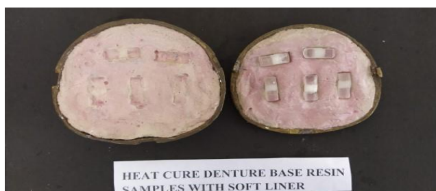
Figure 4 : Heat Cured Denture Base Resin samples relined with Soft liners
