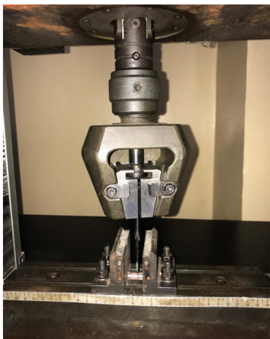
Figure 7 : Shear Bond strength Test
