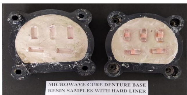
Figure 3 : Microwave Cured Denture Base Resin samples relined with Hard liners
