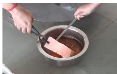
Fig.1.2 Dipping of heated Rajata in liquid media
