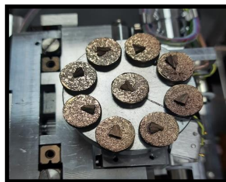
Fig 3- Gold sputtering of the samples
