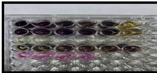
Figure (8): The 96-well plates that contained DMSO with different degree of yellow and purple colors depending on cells viability after the incubation
