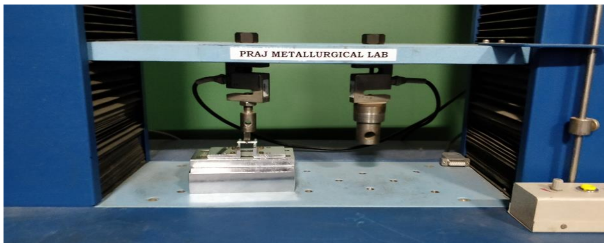
IMAGE 3B :UNIVERSAL TESTING MACHINE FOR FLEXURAL STRENGTH
