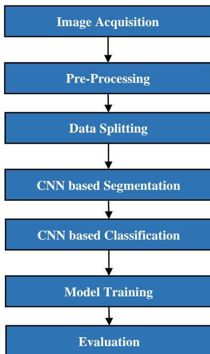
Fig. 2. Flow diagram for proposed road crack detection
