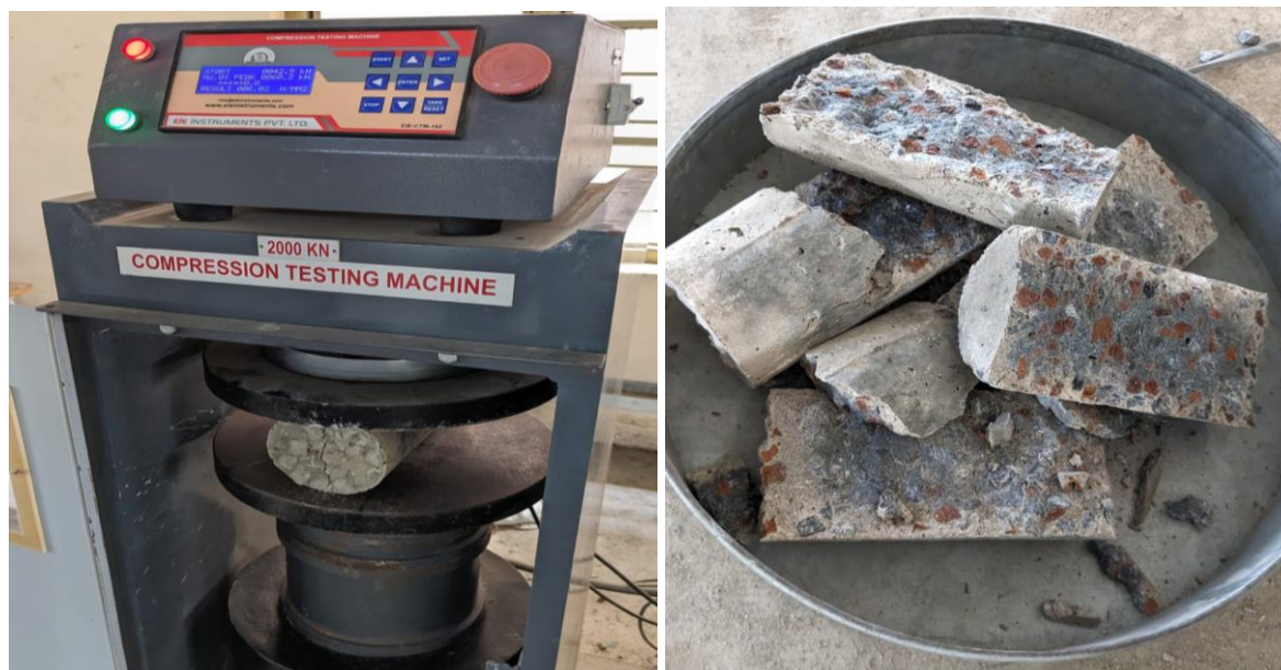
Fig: split tensile strength setup a) test setup using CTM b) after test samples
