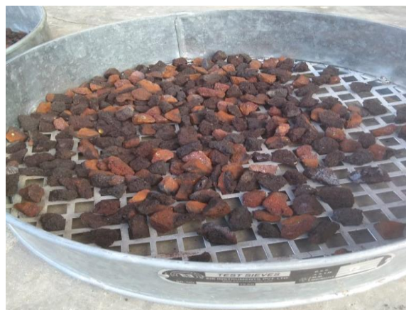
Figure 1: overburnt bricks with the size of coarse aggregates
