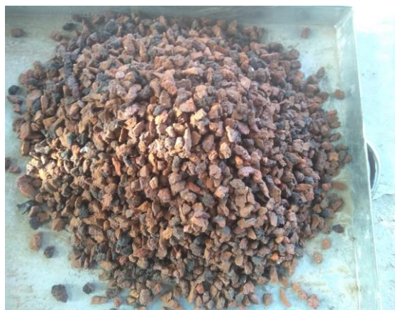
Figure 1: overburnt bricks with the size of coarse aggregates
