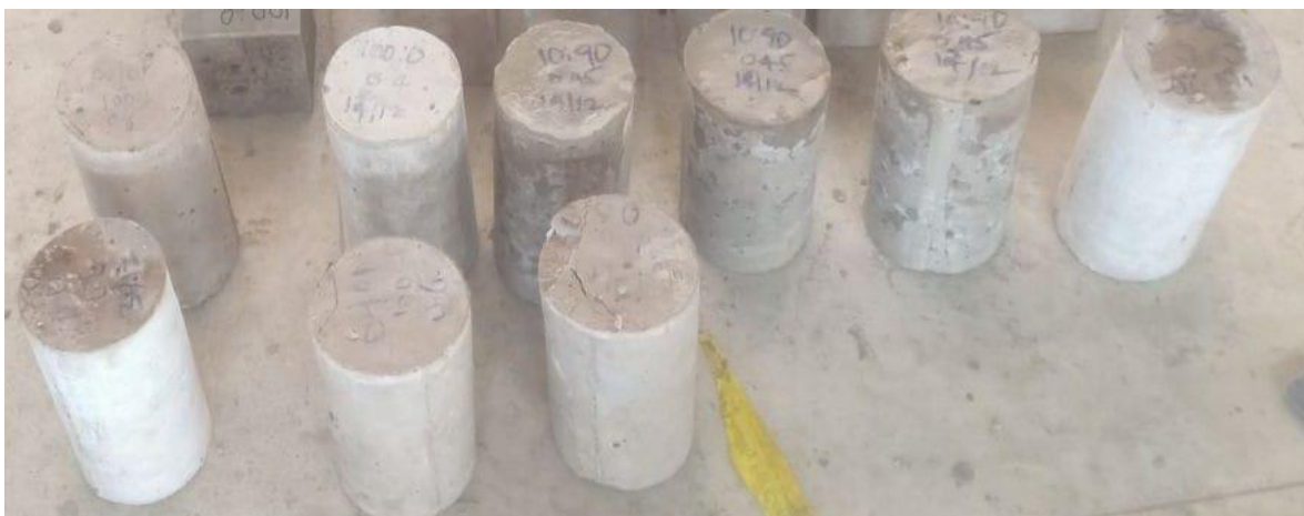
Figure: cylinders (size 100X200mm) for self-curing.
