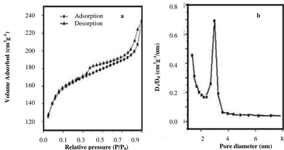
Figure 5. (a) Nitrogen adsorption-desorption isotherms and (b) Pore size distribution of the  $\text{Fe}_3\text{O}_4\text{@MCM-41}$  [25].
