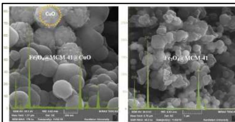
Figure 3. SEM images and EDX spectra of core-shells.
