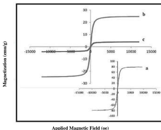
Figure 6. Hysteresis loops recorded of (a)  $\text{Fe}_3\text{O}_4$ , (b)  $\text{Fe}_3\text{O}_4\text{@MCM-41}$  and  $\text{Fe}_3\text{O}_4\text{@MCM41/CuO}$  from solution under an external magnetic field.
