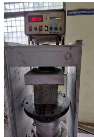
Fig 6 Testing on Compression testing machine
