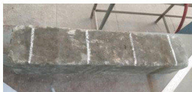
Fig 11 Beam marking for determining flexural strength test
