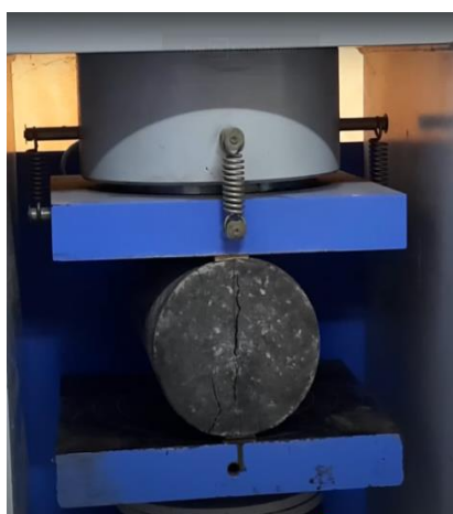
Fig 8 Testing of split tensile strength
