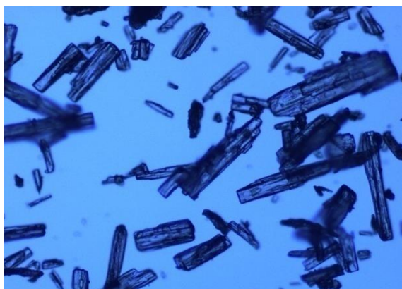
Figure 5: Optical micrographs of optimized batch of co-processed mannitol and MCC
