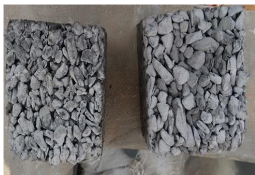
Fig 4.10 Pervious concrete block after curing period
