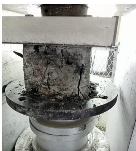
Fig. 8 Compressive Strength Test
