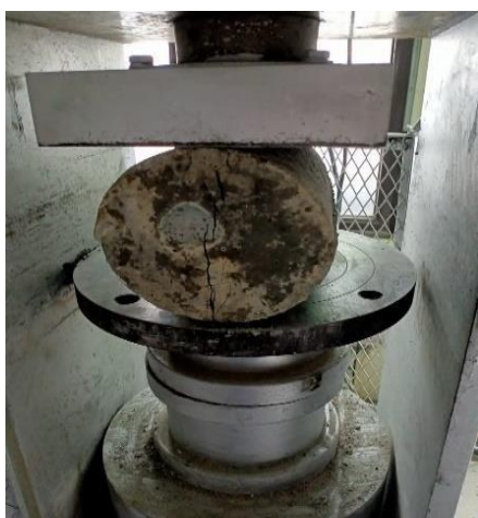
Fig. 9 Splitting tensile strength
