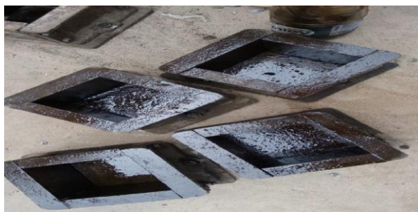
Figure 1. Moulds (150mmx 150mm x 150mm)
