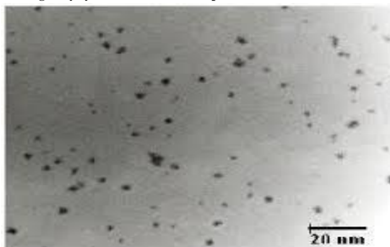
Fig.4 TEM result of the biologically synthesized silver nanoparticles from the bark extract of B.Variegata
