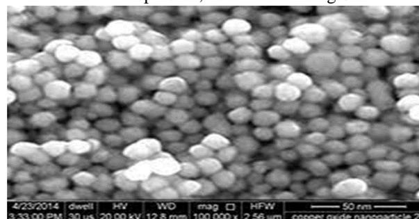
Fig. 3 High resolution scanning electron microscopic (SEM) image of copper oxide nanoparticles (CuONPs). polydispersed (Cluster) CuO NPs ranged between 86.24 - 94.44 nm
