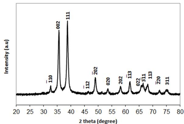
**Fig. 5** XRD patterns of copper nanoparticles synthesized using leaves
