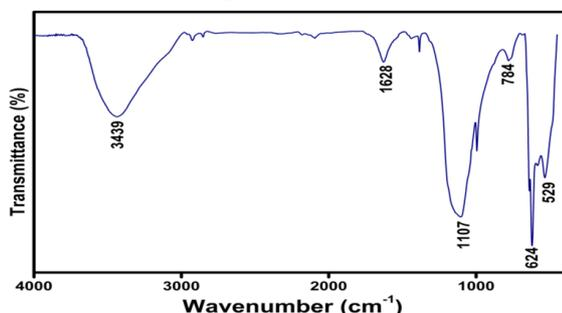
Fig. 2 FTIR spectrum of copper oxide nanoparticles synthesized by reduction of Cu<sup>+</sup> ions by *Mangifera indica* leaves extract
