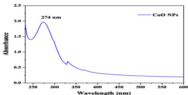
Fig. 1 UV-Vis Spectral analysis of CuONPs
