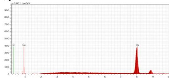
**Fig. 4** EDS-spectroscopy view of the *Mangifera indica* showing synthesis of copper oxide nanoparticles and elemental copper signal in higher percentage
