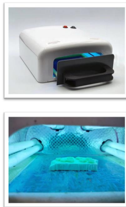
Figure 5. (a) UV light box for light-curing, (b) glazed samples during polymerization
