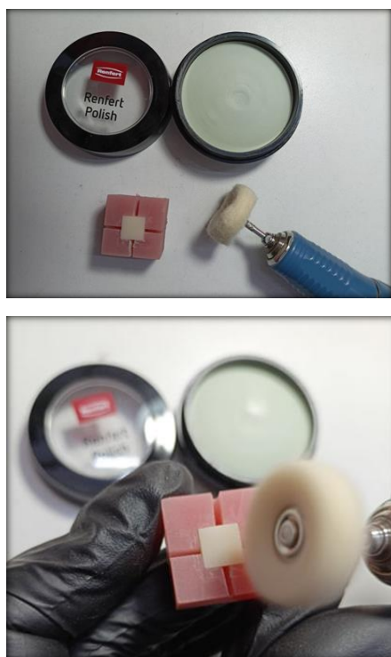
Figure 4. (a) polishing kit and diamond paste, (b) during polishing
