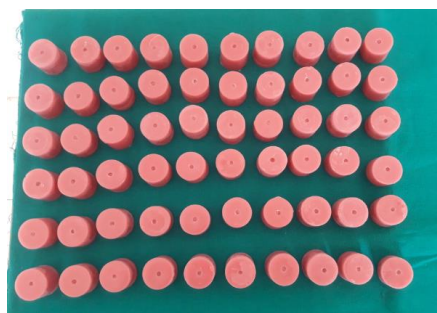
Figure 1: 60 acrylic cylindrical blocks with a central hole of 4mm diameter and 2mm depth
