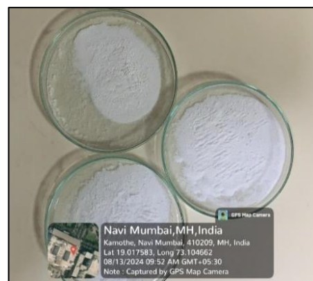
Figure 3: In-House chemically synthesized Al 2 O 3 NPs
