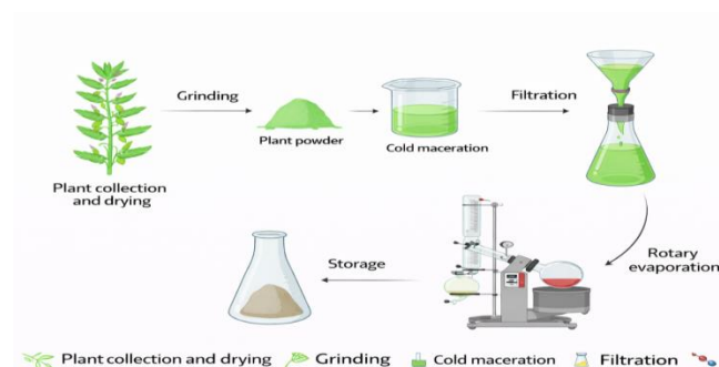
Fig.13 schematic diagram of a plant extraction process using cold maceration
