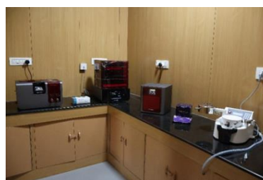
Figure 1. In-office aligner workstation with SprintRay® printing, washing, and curing units.
