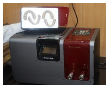
Figure 5. Orthodontic models printed using Taglus® Model resin -washed in the SprintRay® automated washer unit
