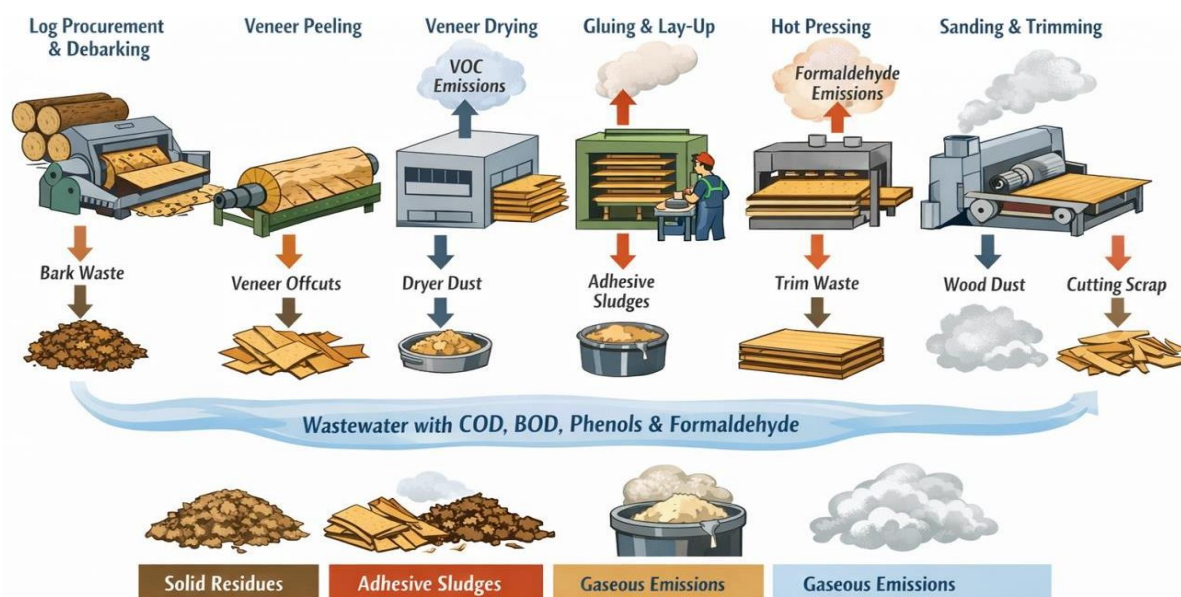
Figure 2. Schematic of plywood manufacturing steps and associated waste streams (solid residues, wastewater, gaseous emissions, adhesive sludges).
