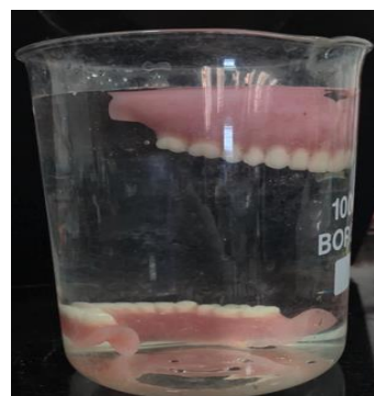
Figure 6. Evaluation for leakage using a water test to confirm the integrity of the hollow cavity.
