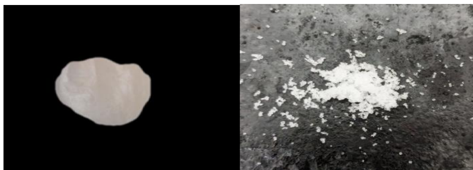
Figure 2: The light cured nanoparticle incorporated composite block and its powdered form (from left to right)
