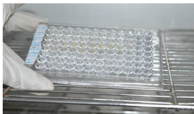
Fig. 2 - Samples from their respective groups were placed in the labeled wells by using a forcep and microtitre plate was incubated at 37 degree Celsius for 24 hours.
