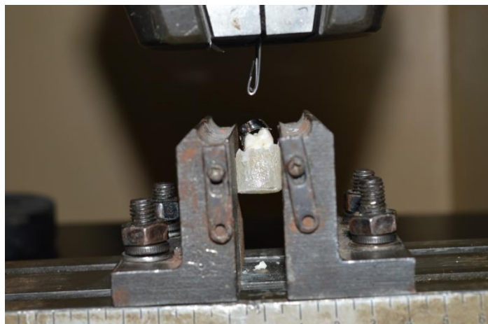
Fig 6 - The maximum load necessary to deband was recorded using the instron testing machine.
