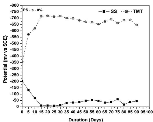
**Fig 5.1** Potential time behaviour of rebars in cement extracts (CE)
