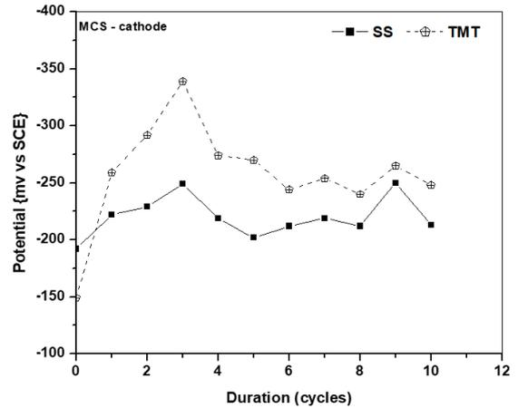
Fig 5.6 Potential time behaviour of cathode rebars
