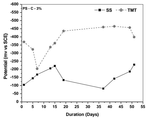
Fig 5.4 Potential time behaviour of rebars in 3%NaCl
