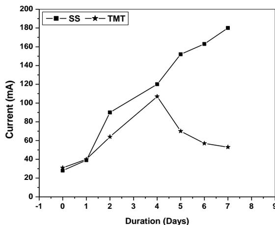
**Fig 5.7** Corrosion current from time to cracking study
