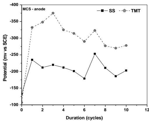
Fig 5.5 Potential time behaviour of anode rebars
