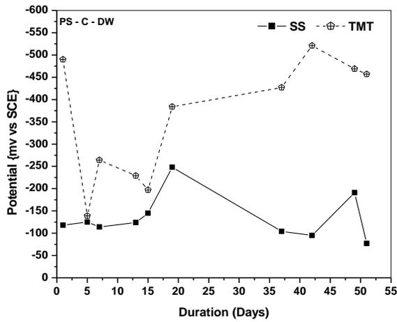
Fig 5.3 Potential time behaviour of rebars in distilled water
