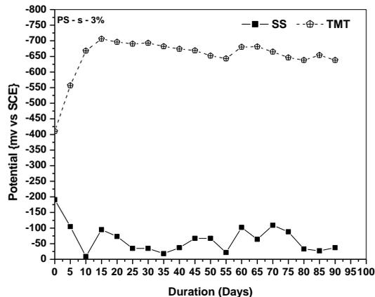
**Fig 5.2** Potential time behaviour of rebars in cement extract and chloride (CE+CL)
